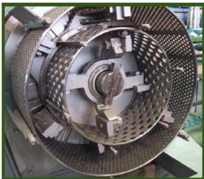
Internal view of the doble grid hammer crusher
